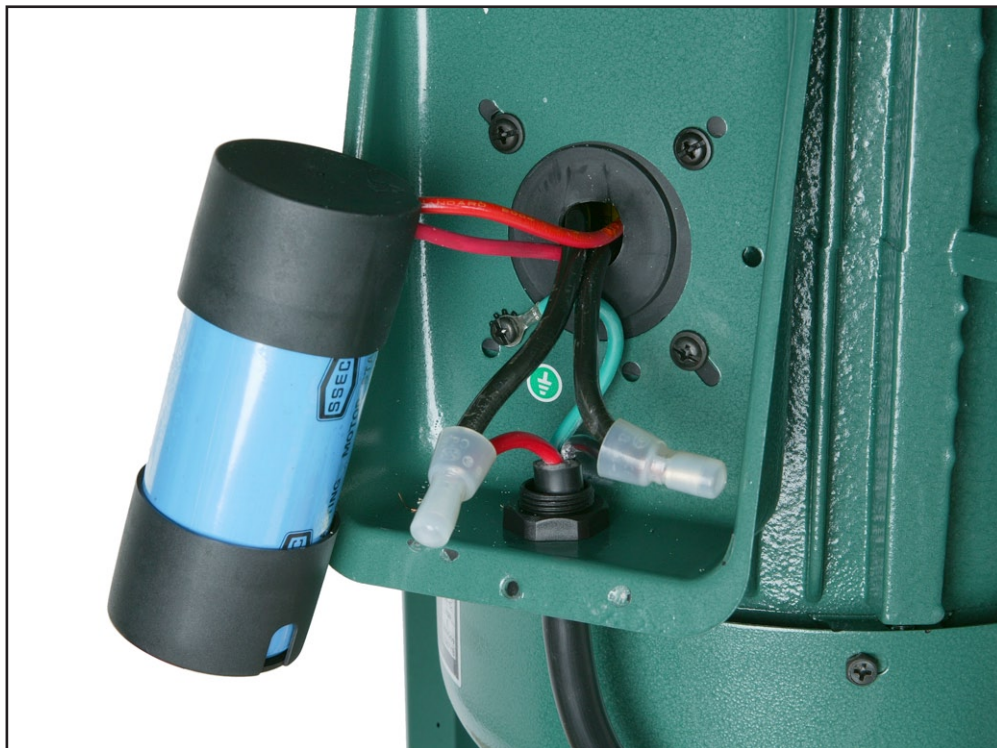
Figure 32. Model G5954 Junction Box Wiring.
